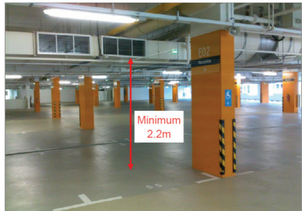
Figure A-23 Example of minimum headroom clearance
